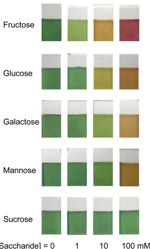
Figure 8. Comparison of responsiveness against various saccharides. The measurement conditions are the same as those in Figure 3. [Color figure can be viewed in the online issue, which is available at wileyonlinelibrary.com .]
